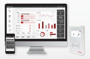
The cloud platform pironex-iot.de and the associated Android and iOS apps enable remote access and offer extended visualization options.
