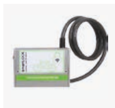
piSmart-Lock (Bike lock with Bluetooth LE and RFID reader)
